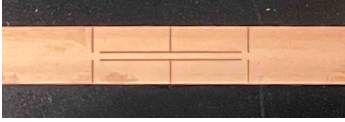
FIG. 61. 0.5 mm wide, 10 mm long bridge on 4 mm wide REBCO sample from SST. The lobes above and below the bridge can be used for voltage taps.
