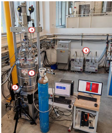
FIG. 96. View of the system installed at the Institut Clément Ader, (1) cryostat, (2) CCD camera, (3) test stand, and (4) cryo-cooler compressors.
