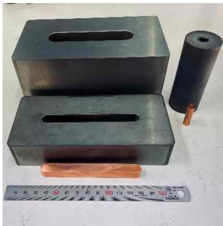
FIG. 114. Photograph of the 8 mm diameter SPS cylinder and its die (right), the 10 \times 10 \times 100 \text{ mm}^3 SPS bar and its die (bottom left), the SPS die for future 20 \times 20 \times 100 \text{ mm}^3 samples (top left).
