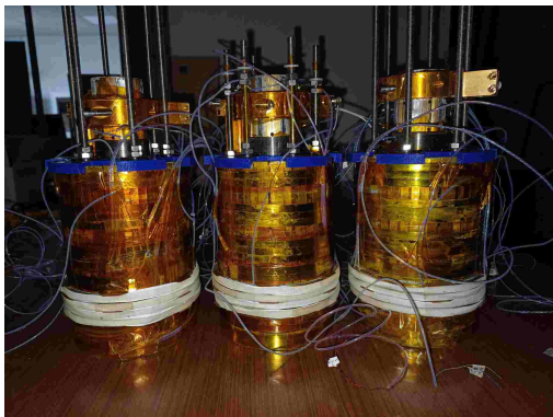
FIG. 67. MI HTS mock up coils made of a stack of two double pancakes to test in-situ the HTS tapes close to their operating condition at 4.2 K in magnetic field background up to 20 T.
