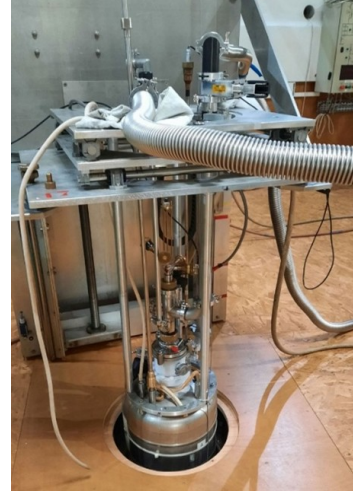
FIG. 99. User platform of the 42 T hybrid magnet showing the xy -table which supports a ^4\text{He} bath cryostat with a ^3\text{He} insert and NMR probe. Vacuum tubes for ^4\text{He} and ^3\text{He} bath pumping are also visible. The magnetic field center is \simeq 1.8 m below the wooden platform. The cold bore diameter is 16 mm for a room temperature magnet bore diameter of 34 mm. As seen, the cryostat is raised by about 1 m with respect to its position during scientific experiments.
