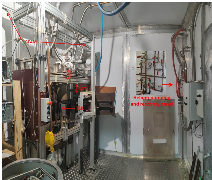
FIG. 98. The MegaGauss workstation arrangement showing the helium pumping and recovery system.
