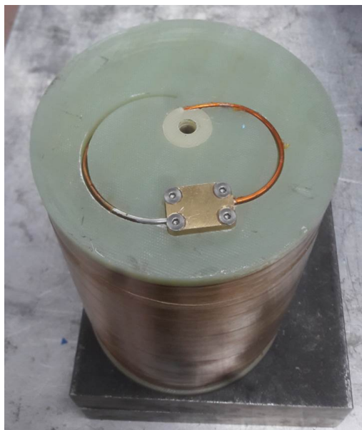
FIG. 125. The first bi-material inner coil prototype showing the output of the 3rd layer of Cu-Nb (right) connected by a brass junction to the entry of the 1st layer of Cu-SS (left).
