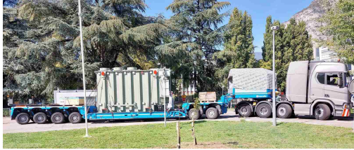
FIG. 101. 28th of September 2023; arrival of the new 60 MVA 225 kV/15 kV from SIEMENS-Italy through the Frejus Tunnel.
