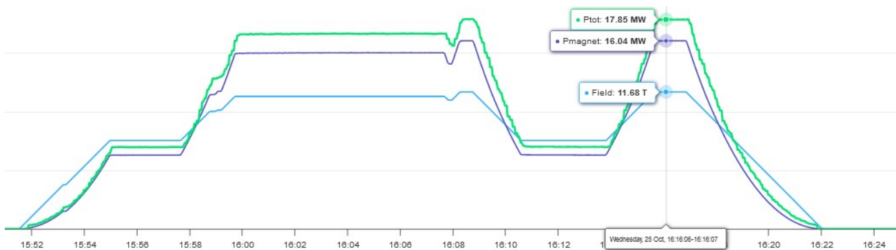
FIG. 103. Qualification test for 30 MW operation. Chronogram of the 25th of October 2023. Blue: Magnetic Field, Purple: Power on the bitter coils, Green: total Power. The high field magnets are made of two submagnets powered and cooled independently (only the low pressure cooling side is in common). Powering a 30 MW magnet will consist of powering one submagnet at 18 MW and the other one at 12 MW.
