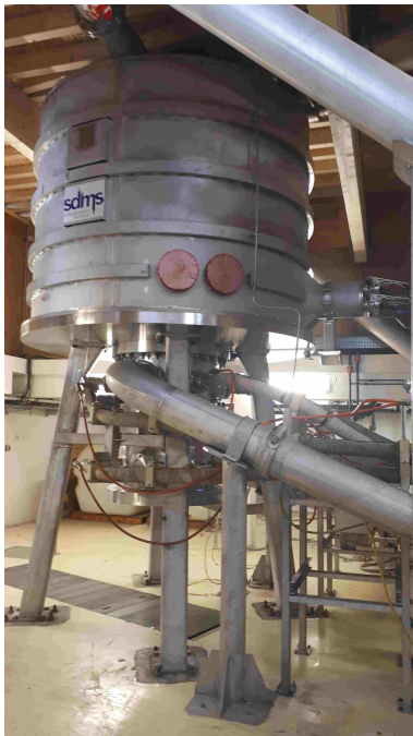
FIG. 110. View of the hybrid magnet from the ground floor. The total height is about 5.4 m for a total weight of about 52 tons. Water cooling system for the 24 MW resistive inserts can also be seen.
